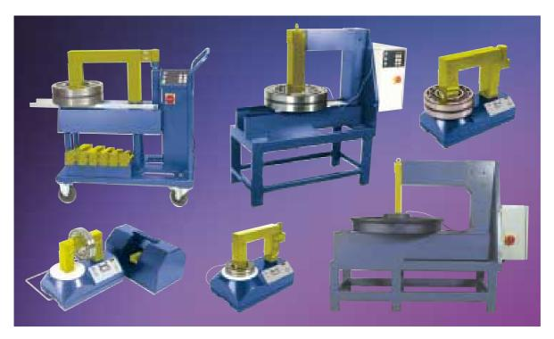
Heat assisted installation consists of thermally expanding the bearing by raising the temperature, then sliding it onto the shaft without the need to apply force.
