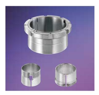
Adapter sleeves produce an interference fit between bearing and rotating shaft by pressing the bearing onto the sleeve. Withdrawal sleeves allow easy removal by simply screwing in the extraction nut (pushing the sleeve into the bearing bore). To facilitate large-size bearing installation and removal, SNR has also developed a range of hydraulic sleeves.
